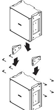
Then, fix the GH-FLY bar to the speaker's GH-FLY frame with the provided pins, adjusting the bumper to achieve the desired height and angle, and suspend the array in vertical to the rigging point.
